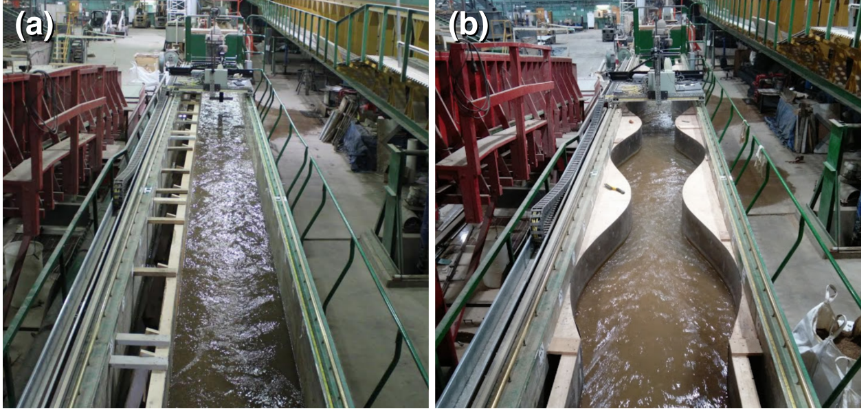
Figure 4.2: (a) Straight-walled flume geometry and (b) variable-width flume geometry. Camera view is oriented downstream in both images.
