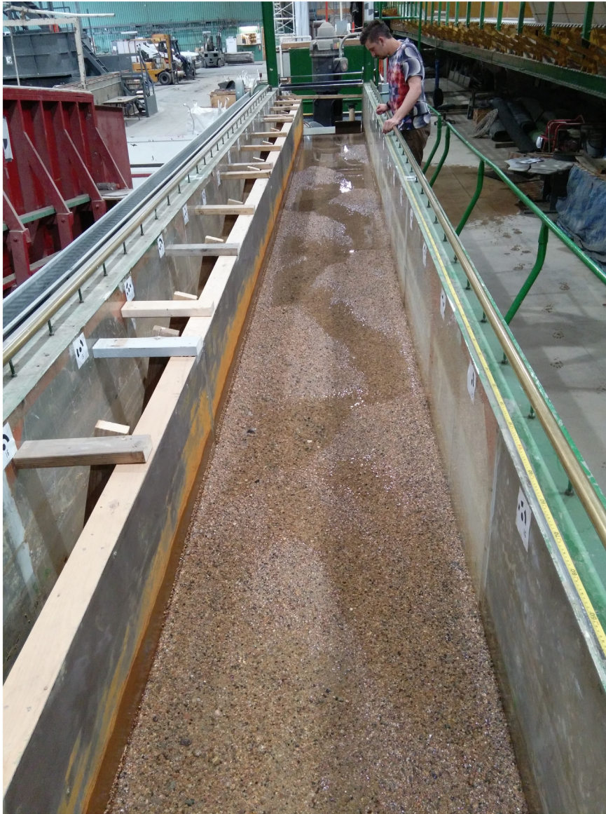
Fig. 5. Photograph of the flume as it was draining, illustrating the alternate bars that developed. View is looking downstream.
